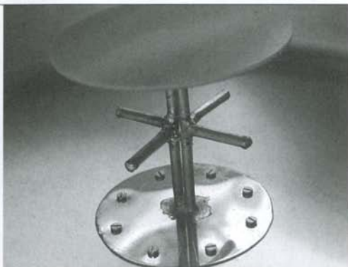
Fig. 9 Feed for circular polarization and its dimensions (rear view: the field is propagating inside the sketch; measures in mm). The length of each dipole is a critical parameter for reaching almost circular polarization. The tuning had been made soldering little patches to the ends of the dipoles and testing the circularity using the standard gain antenna shown in fig. 15.
